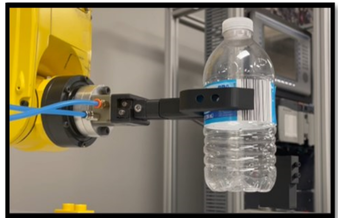
Figure 16. Two-inch gripper holding a 10 oz. water bottle.
