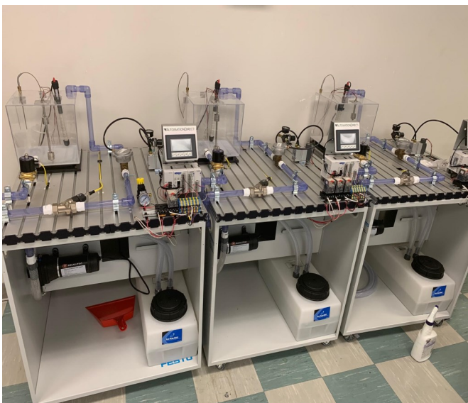
Figure 1. The complete industrial instrumentation trainers built by the students.
